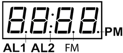
AL1 indicator is ON when Alarm 1 is on.
