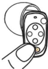
**To turn the hearing aids off:** Press and hold the button on the side of each hearing aid **for 6 seconds**. After 3 seconds, you'll hear the program change beeps—**KEEP PRESSING** until you hear a long beep, which signals the hearing aid is turning off.
