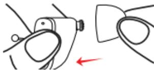
2. Pull gently on the dome to make sure it's secure. Then push the flaps of the dome back into place.
