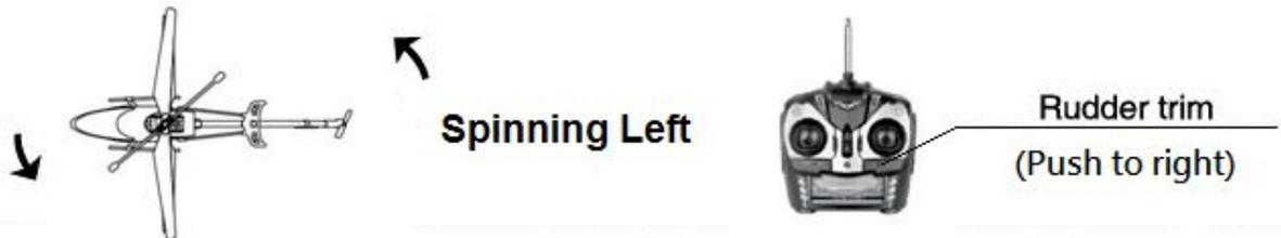
When the helicopter spins right excessively, push the rudder trim to left slowly until the helicopter stops spinning.
